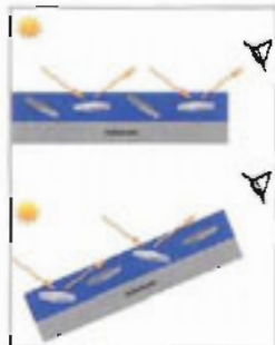
Figure 3: Sparkle effects are created when different pigment particles come into line (see note - 2)
