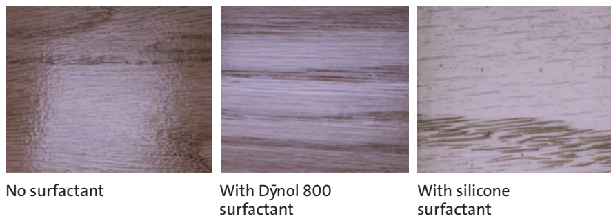
Figure 8: Brush applied wood coating
