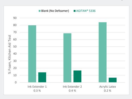
AGITAN® 5336 provides excellent defoaming across a variety of aqueous formulations in medium- to high-shear testing, at the same levels used for typical mineral oil defoamers.
