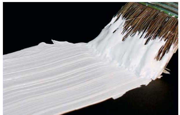
Figure 1 | Annoying brush marks in the application of a wall paint.
