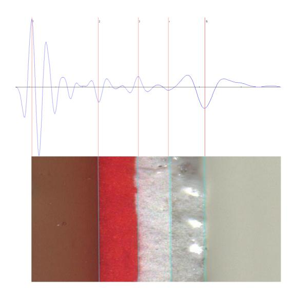
Typical ultrasonic echoes generated by paint layers:
