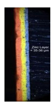
On this sample, the substrate is smooth, and the zinc prime layer is uniform in thickness.
