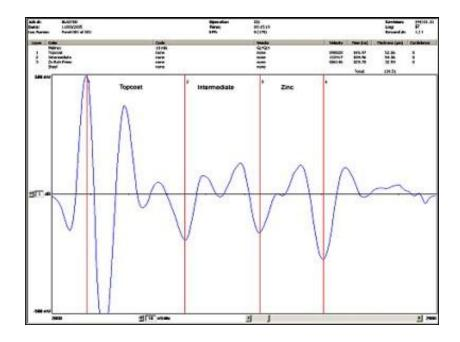
Despite the blasted substrate, the echoes are clear with clear layer boundaries, resulting in accurate thickness measurements.
