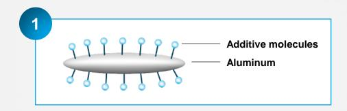
Adsorption of corrosion inhibitors on the active surface of the pigment surface (additive technology)
