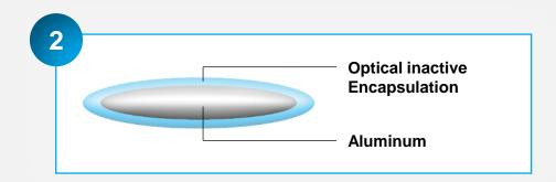
Encapsulation of the aluminum pigments with metal oxides or a transparent silica layer (encapsulation technology)
