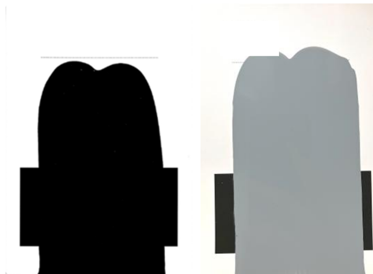
Comparison of liquid colorant (left in drawdowns) and solid colorant (right in drawdowns)
