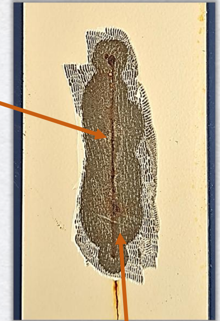
Clean metal under coating High adhesion
