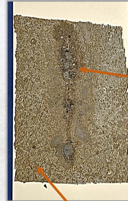
Corroded metal under coating Adhesion loss
