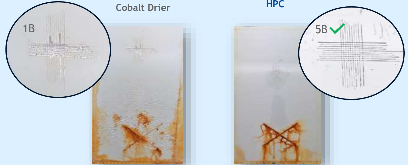
Wet cross-hatch rating (after 300 hrs Q-FOG) Corrosion panels after 330 h in Q-Fog
