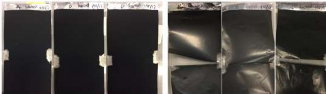
All the powders were well attached to the substrate after electrostatic spraying.
