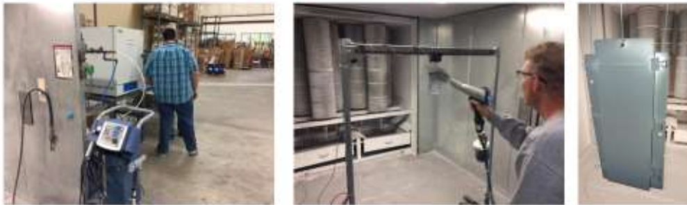
Collaborators at Keyland Polymer are evaluating electrostatic spraying method for battery coatings.
