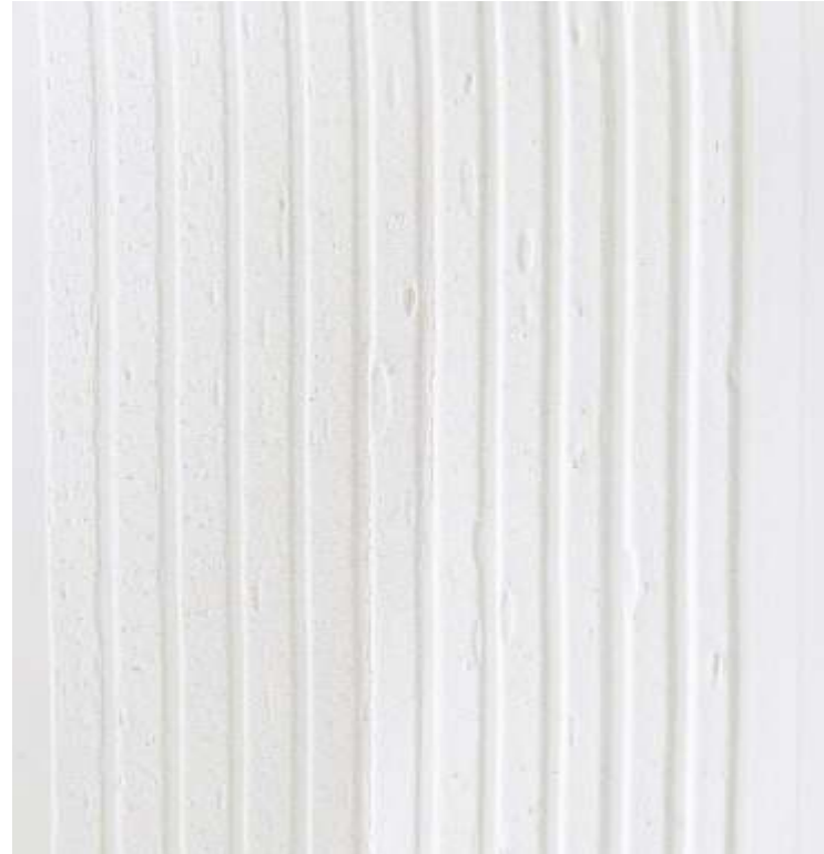
MFC (3.80 w-% of 10% MFC) No Cracking, Pass 60 Mils (1.52 mm)
