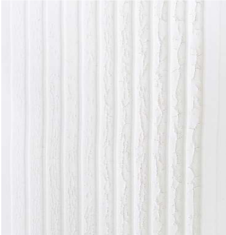
Reference with HEC (0.31 w-%) Cracking > 14 Mils (0.36 mm)
