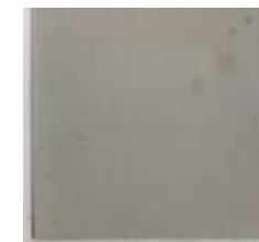
Formulation with adhesion promoter after 2 weeks @ 85°C/85%RH
