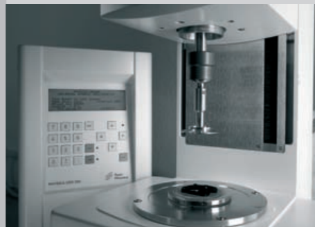
1995 Introduction of Physica UDS 200 – First rheometer with EC motor (brushless DC)
