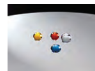
Water droplets on silicon wafer treated with SIH5841.5 exhibit high contact angle
