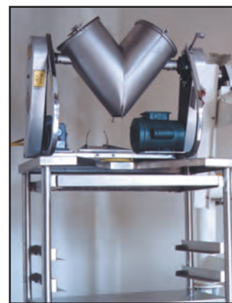
Fig. 3 Twin-cone blenders with intensive mixing bars are used for bulk deposition of silanes onto powders.
