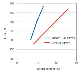
Compressive load as function of polymer content for Boltorn<sup>™</sup> H311 vs. co-polymer polyols
