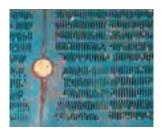
Polyester adipate-based end products show less durability in withstanding a harsh environment and, as seen above, this can lead to rapid deformation
