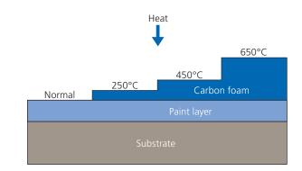
Charmor<sup>TM</sup> extends the time it takes for steel to reach the critical temperature of  $500^{\circ}C$
