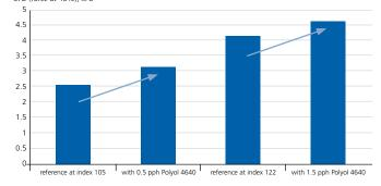
Hardness improvement in 20 kg/m³ density TDI flexible foam with addition of 0.5 to 1.5 parts of Polyol 4640
