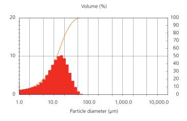
Particle size distribution of Charmor<sup>™</sup> PM40 Typically 98% of particles are below 40 µm
