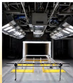
Atlas Custom Systems designs and builds custom solar simulation systems such as walk-in chambers or full-scale test facilities. These full scale test facilities use a series of highly coordinated metal halide lights to provide uniform radiant energy to meet the demanding testing needs of many industries.
